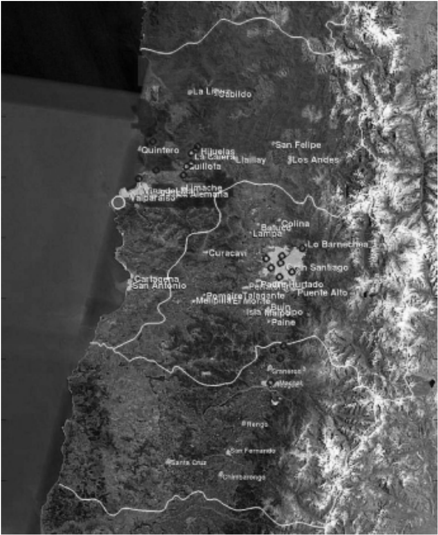
FIGURE 3.5 Influence of a large power plant on ozone formation, calculated as the difference between modeled ozone with and without emissions from the source. Light shading denotes an increase in ozone concentration greater than 1\text{ }\mu\text{g}/\text{m}^3 ; dark shading denotes a decrease in ozone concentrations. The dot denotes the location of the point source. WRF-Chem at 3 km resolution was used.
